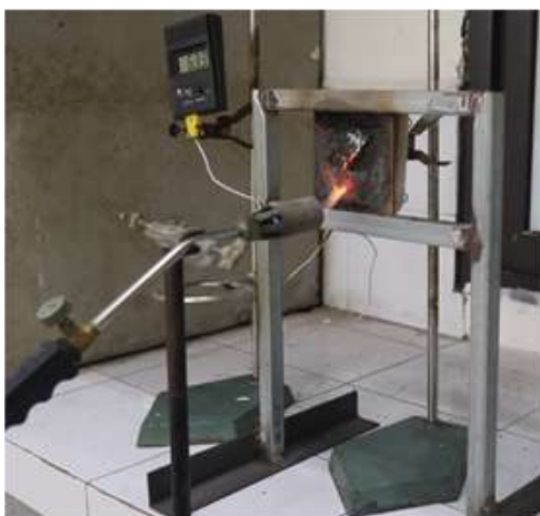
Figure 1. Experimental setup for testing fire performance of intumescent coatings
