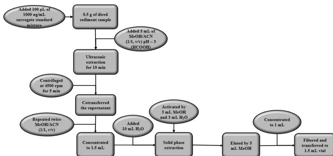
Figure 3. The optimized procedure for sediment sample treatment.
