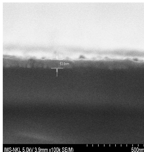
Figure 5. SEM images of the SERS-based AuNP layer, showing cross-sectional thickness on a glass substrate prepared via drop-casting.
