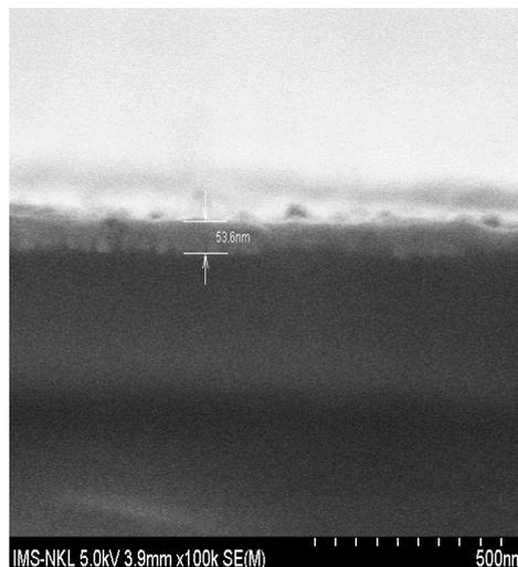
Figure 5. SEM images of the SERS-based AuNP layer, showing cross-sectional thickness on a glass substrate prepared via drop-casting.
